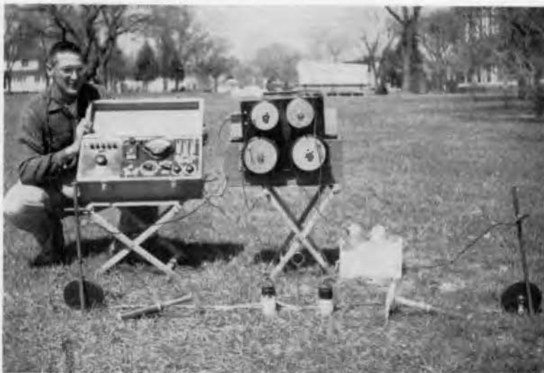
Figure 1. Portable electrical resistivity apparatus used by the Iowa State Highway Commission.
