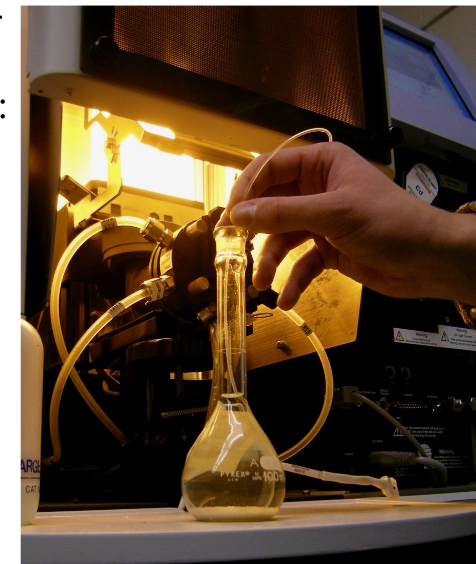
Figure 3: 10000ppm tusk solution being run on the AAS instrument
