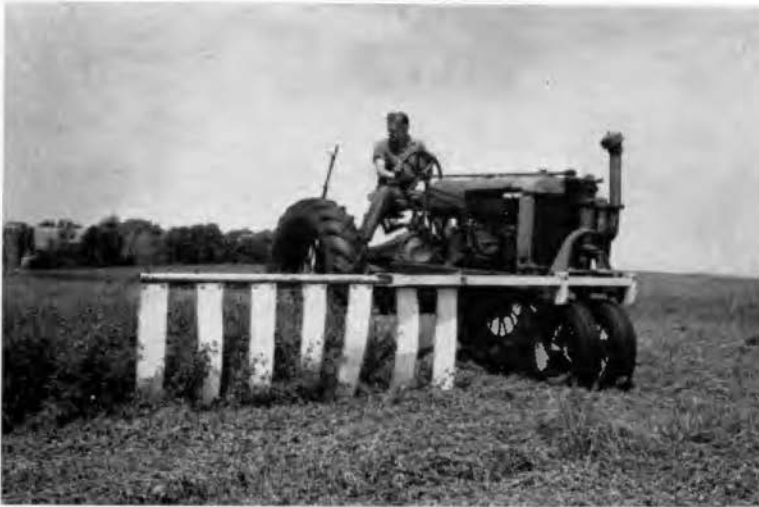
Figure 3. A flushing bar with heavy belting was one of the types tested for effectiveness in scaring pheasant hens ahead of the mower.
