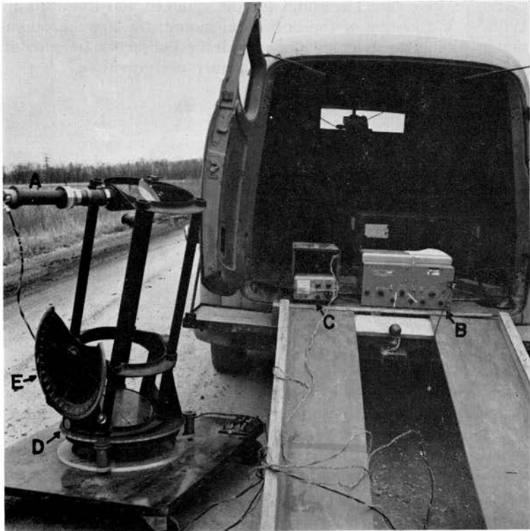
Figure 1. A: Photomultiplier; B: Amplifier-Recorder Unit; C: Power Supply; D: Azimuth Setting-Circle; E: Altitude Setting-Circle.
