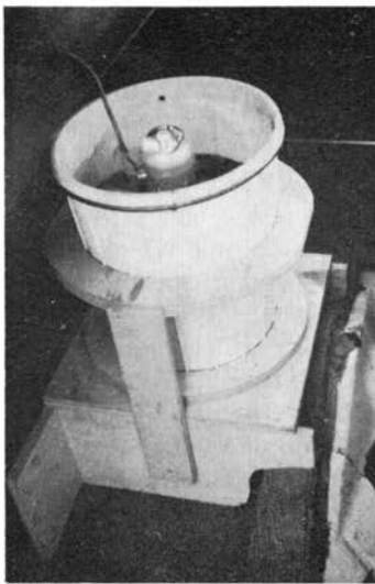
Figure 2. Jalander magnetometer in foam plastic support ring floating in oil-filled container mounted in back seat of automobile.
