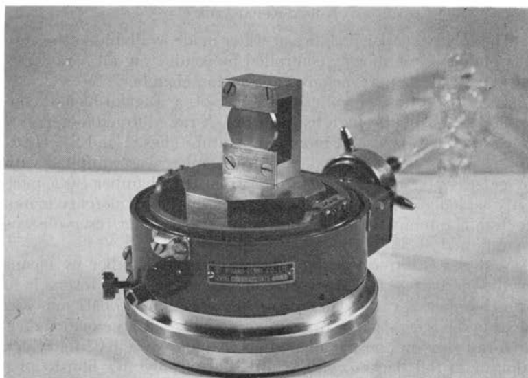
Figure 1. (a) X-ray adsorption apparatus, assembled. (b) Base of the X-ray adsorption apparatus showing the sample holder.
