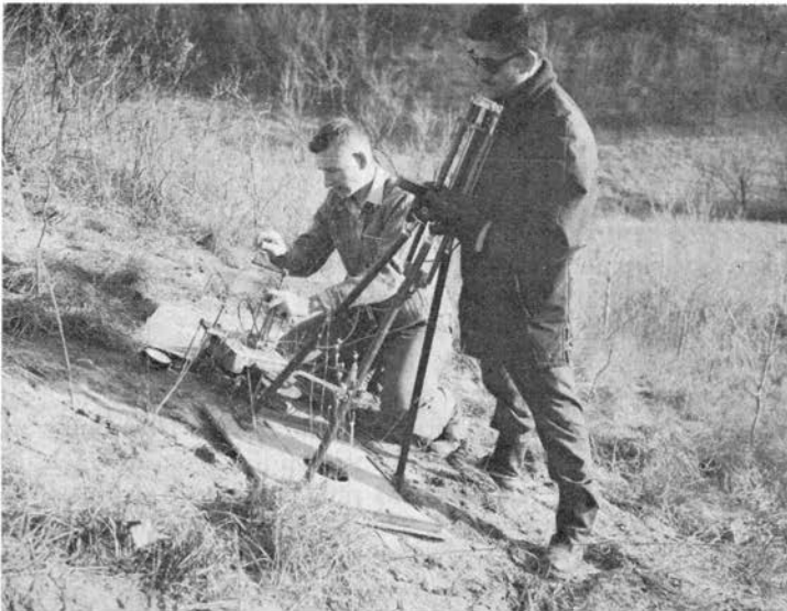
Figure 2. Field set-up for shear test.
