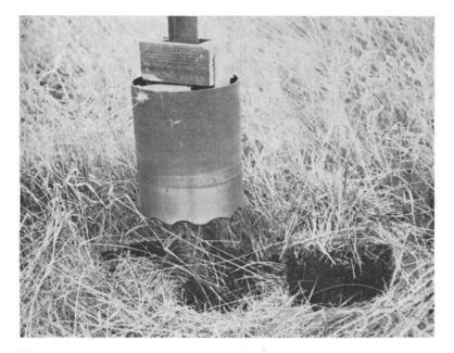
Fig. 1. Sod cutter and sod. Sod is 25cm in diameter.
