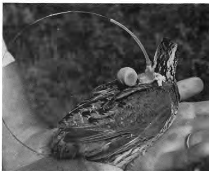
Figure 1. Transmitter and battery.
