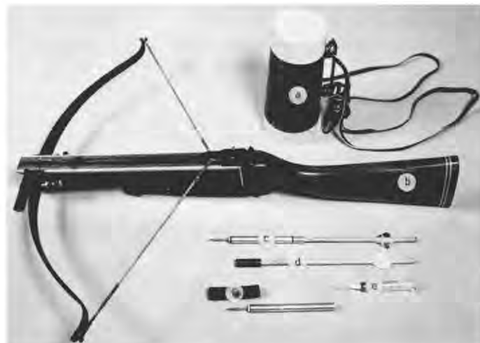
Fig. 1. Immobilizing equipment: a— vacuum bottle for keeping drugs cool and handy in the field; b— crossbow; c— cap-chur dart with fletched wood shaft; d— practice arrow weighted to match loaded dart; e— syringe for administering antagonist; f— rubber hose safety cover (cork in one end) for carrying darts.
