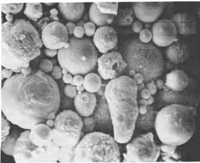
Figure 5. Scanning electron photomicrograph of particles from the magnetic fraction of fly ash, (750 X).
