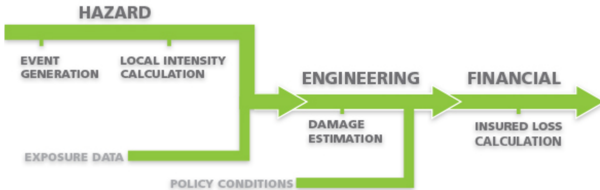
Figure 1. Catastrophe modeling framework. This figure provides a flow chart of the various steps AIR takes when creating a catastrophe model. Adapted from “About Catastrophe Modeling,” by AIR Worldwide, n.d. ( http://www.air-worldwide.com/Models/About-Catastrophe-Modeling/ )
