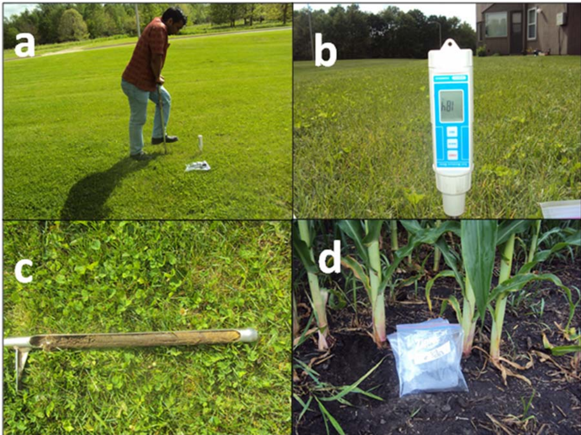
Figure 18. Soil sample collection. a) soil probe, b) digital soil moisture meter, c) a soil profile, and d) soil samples in ziploc bags.
