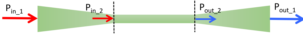
FIGURE 4.10: P_{in2} and P_{out2} refer to the input and output power of the hybrid waveguide as plotted in figure 4.9.
