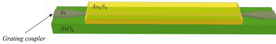
FIGURE 4.5: Schematic of the hybrid waveguide.
