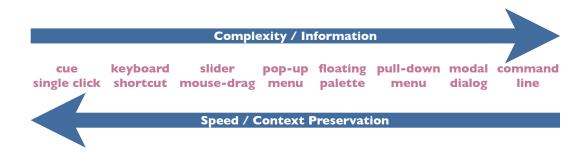
Figure 1: A scale of alternative methods for interactive commands and controls.
