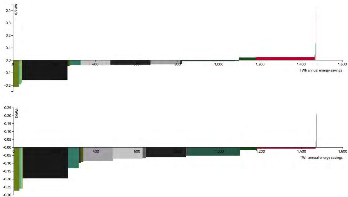
Figure 5. Net marginal energy cost savings (total) by EEI action for EU28 in 2030 (upper graph: excluding and lower graph: including MI) (excluding modal shifts and trucks) (expert mode).
