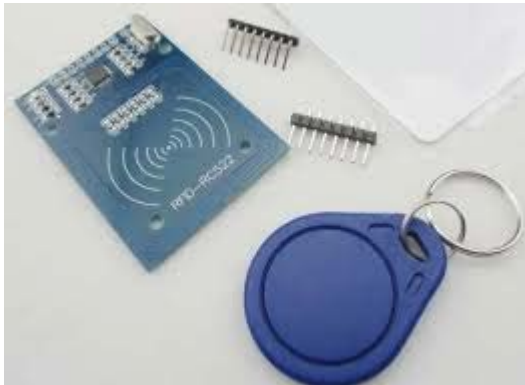
Figure 2-5: Example of an RFID reader on the left, and an RFID tag on the right (LAZADA, 2018)
