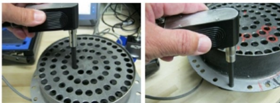
Figure 100: Eddy current testing of DMLS component (Waller et al. , 2014)
