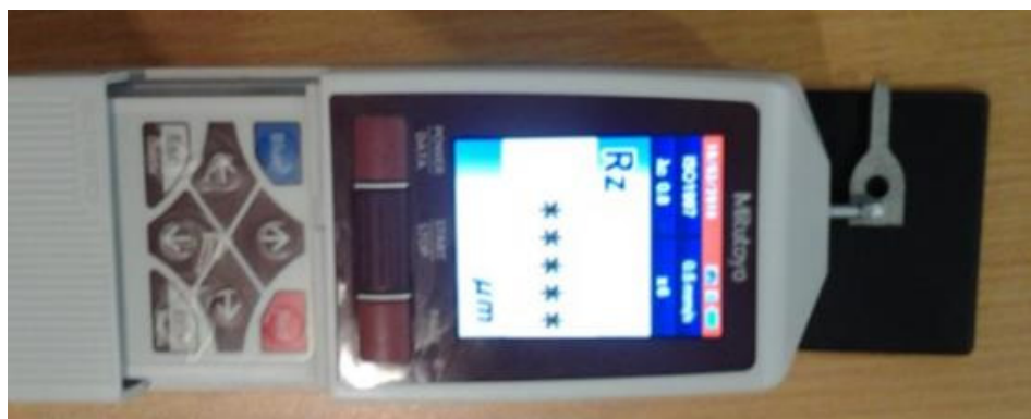
Figure 118 Surface roughness tester SurfTest SJ-210 measuring the flat specimen
