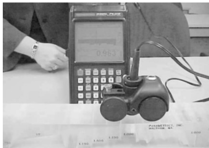
Figure 61: B-scan instrument (Hellier, 2012)
