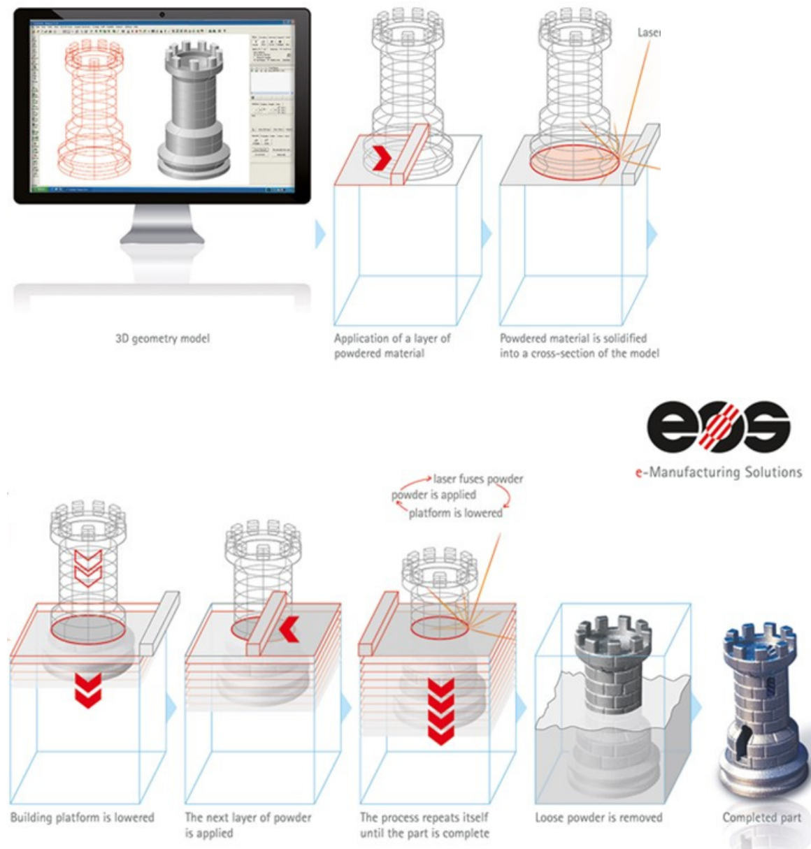
Figure 4: Functional principle of the DMLS (EOS GMBH, 2016)
