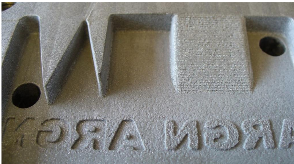
Figure 4.60 Text features and knife-edge corners without any wear after 200 IM cycles using PP.
