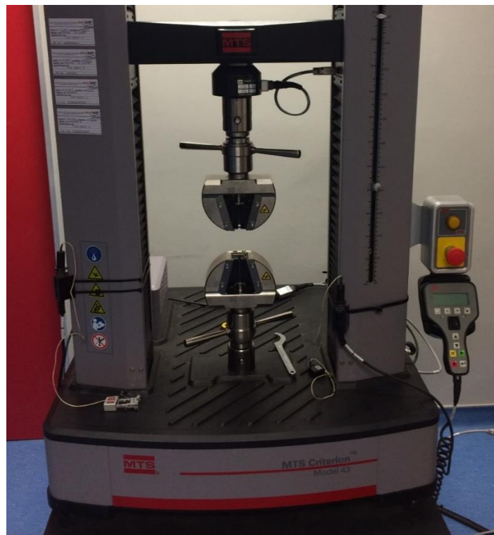
Figure 4.4 MTS Criterion™ Model 43 tensile testing machine used to conduct the tensile testing of the Alumide® test pieces.
