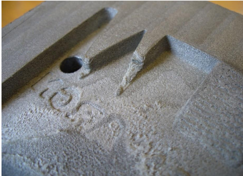
Figure 4.85 Wear of text features and knife-edge corners after 150 IM cycles with PA 6 material.
