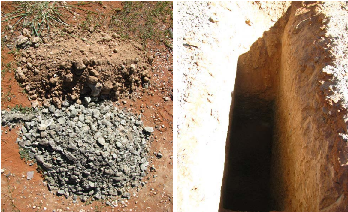
Figure F.10: Test pit 5 materials and test pit
