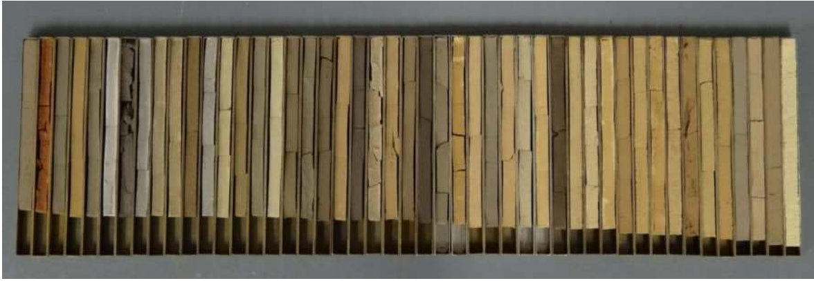
Figure 3.5: Linear shrinkage tests on various samples (Taken from Stott and Theron, 2015)
