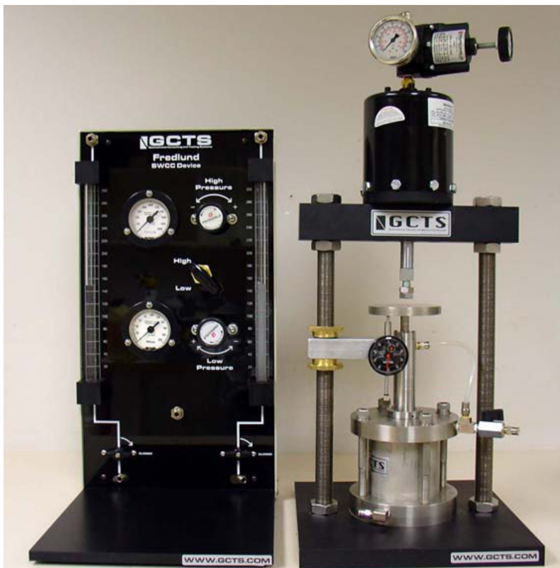
Figure 2.14: Fredlund SWCC device with loading frame (after Chao, 2007)
