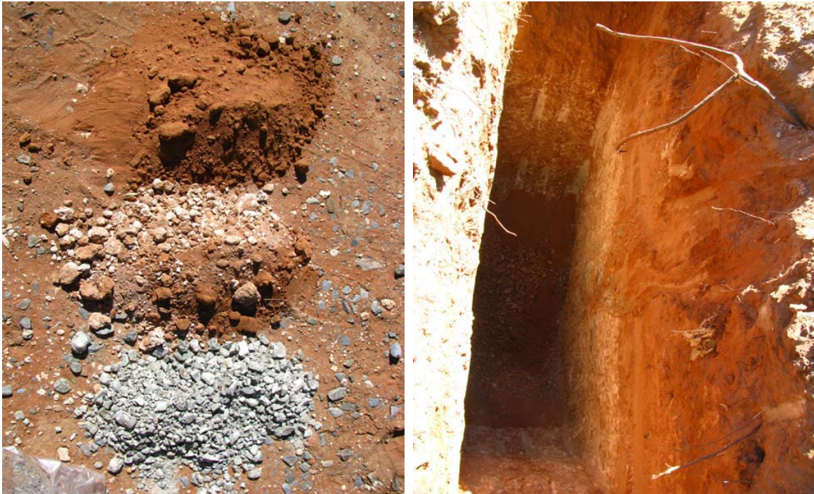
Figure F.9: Test pit 4 materials and test pit
