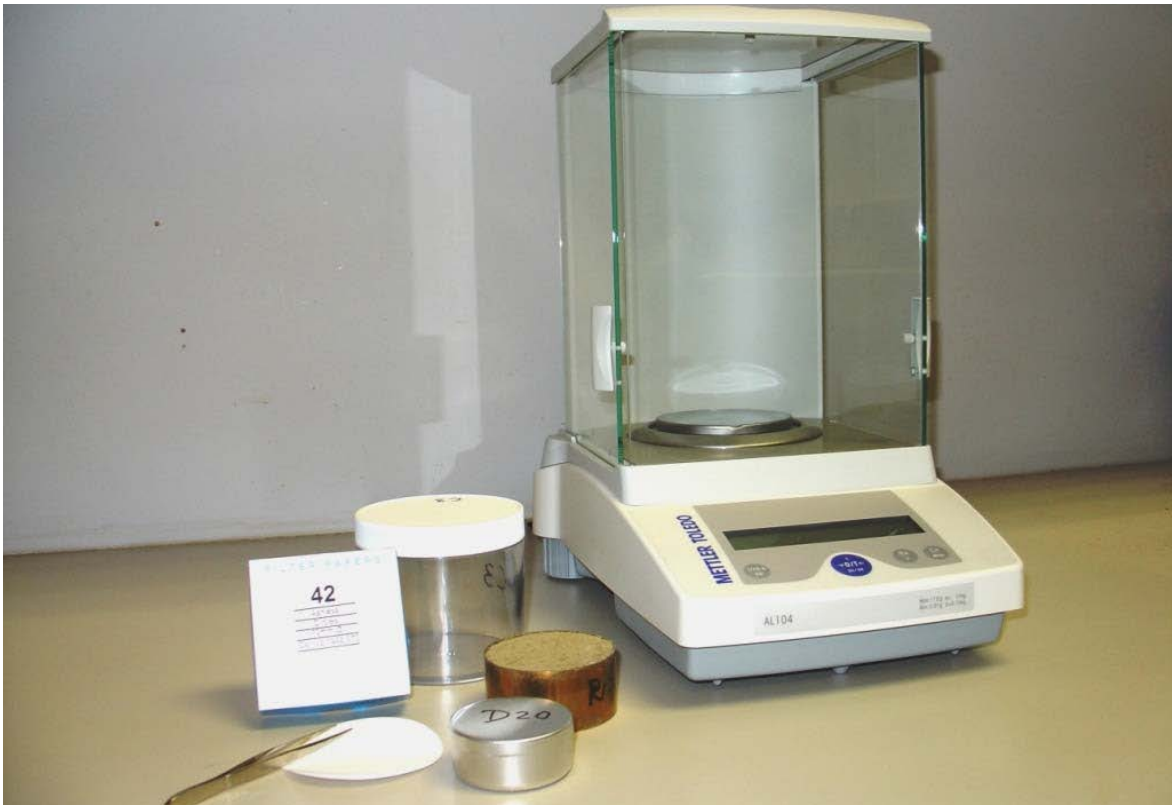
Figure 2.15: Filter paper test equipment, including Whatman® no 42 filter paper (from Chao, 2007)
