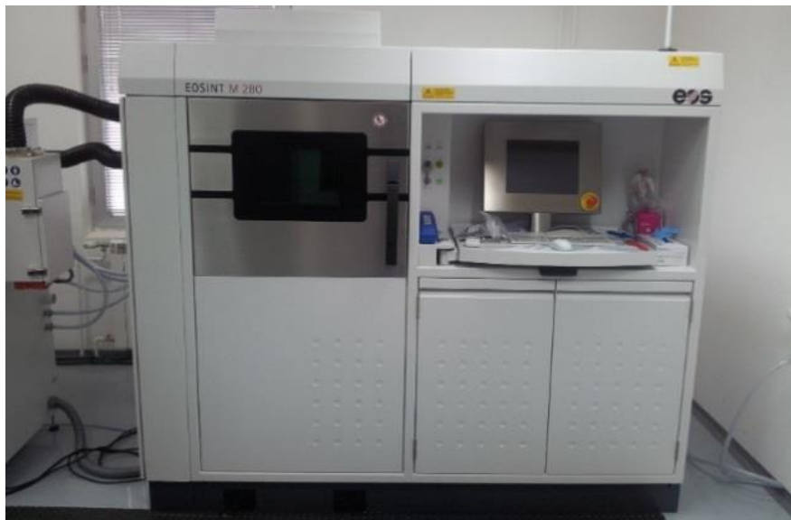
Figure 3.4.1: EOSINT M280 machine installed in CRPM (CUT)
