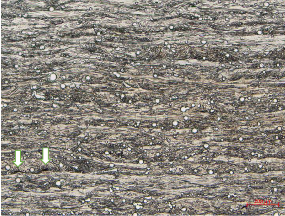
Figure 6.5.6: Interlayer pores (white arrows) in the Ti15Mo microstructure.
