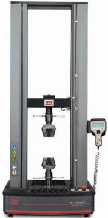
Figure 3.4.7: MTS Criterion model 43 Electromechanical Universal Test Systems machine.
