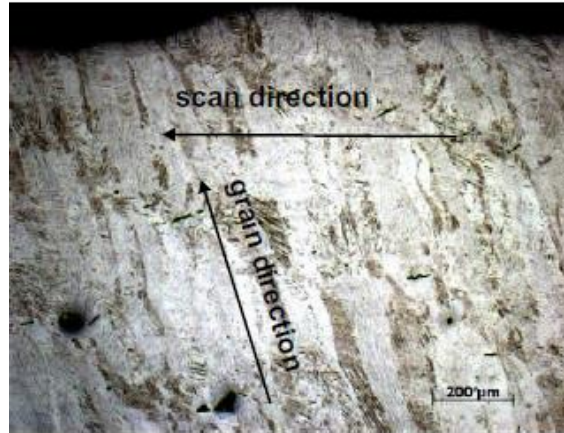
Figure 2.1.18: Influence of scan strategy on the grain direction in Ti6Al4V parts (Thijs et al. , 2010).
