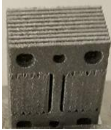
Figure 6.5.8: As-built Ti15Mo mini samples.
