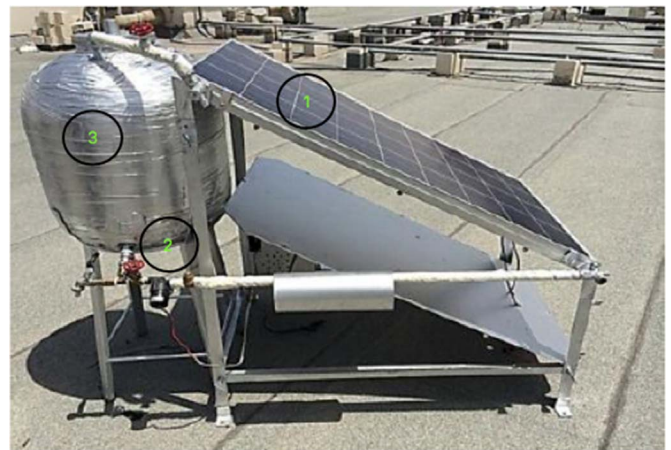
Fig. 6. Hybrid solar Photovoltaic/Thermal (PV/T) cooled by forced water circulation [20].
