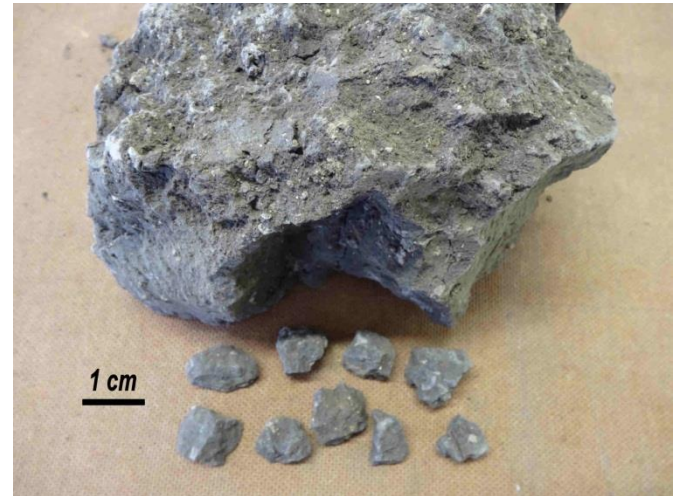
Figure 7 Small samples broken from a small clod of clay
