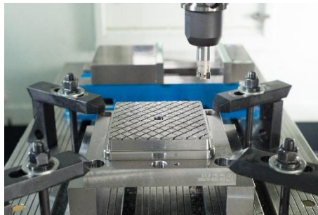
Figure 12: CNC machining of conventional manufactured insert
