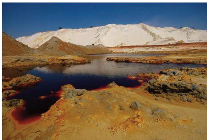
FIG 1. Acid mine drainage generated in surface tailings deposits in the West Rand [53].
