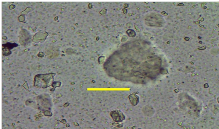
Figure 8.4: Olive grey residual clay treated with dispersant.
