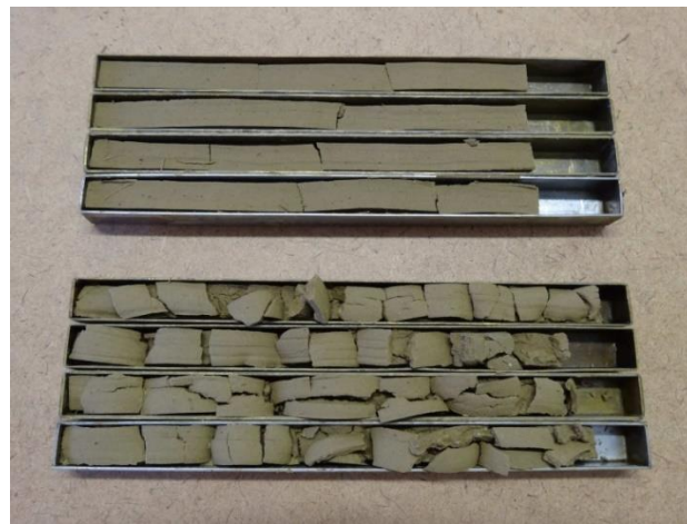
Figure 3.1: Linear Shrinkage of a plastic clay, air – and oven dried.
