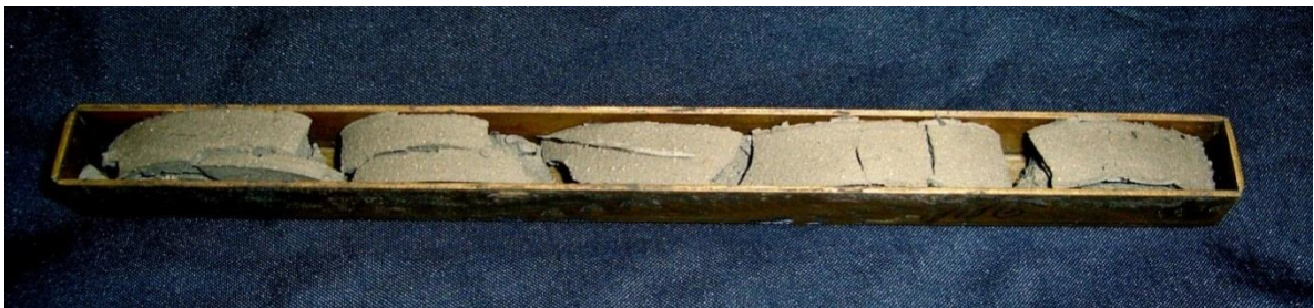
Figure 2.4: Oven-dried sample of firm grey-olive residual clay
