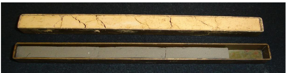
Figure 2.6: Contrasting high and low linear shrinkage.
