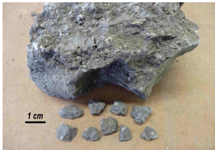
Figure 7.7: Small samples broken from a clod of clay.
