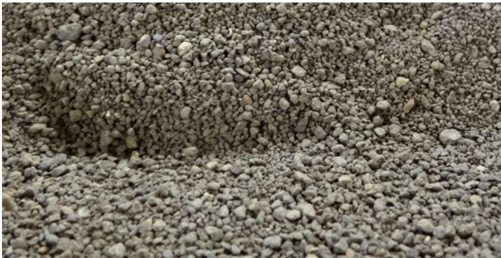
Figure 2.8: Material retained on the 0.425mm sieve.
