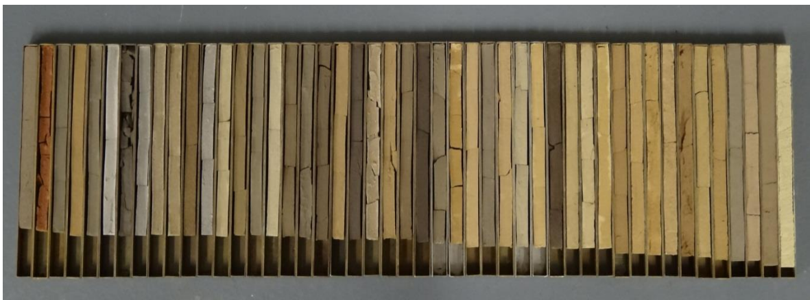
Figure 2.7: Shrinkage troughs with air dried samples.
