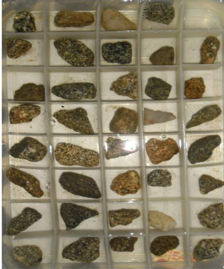
Figure 31 Aggregate after 20 days of ethylene glycol soaking
