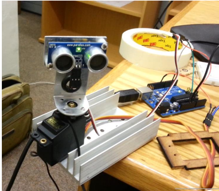
Figure 3-29 Panning Ultrasonic Sensor Mounted to the Servo Motor
