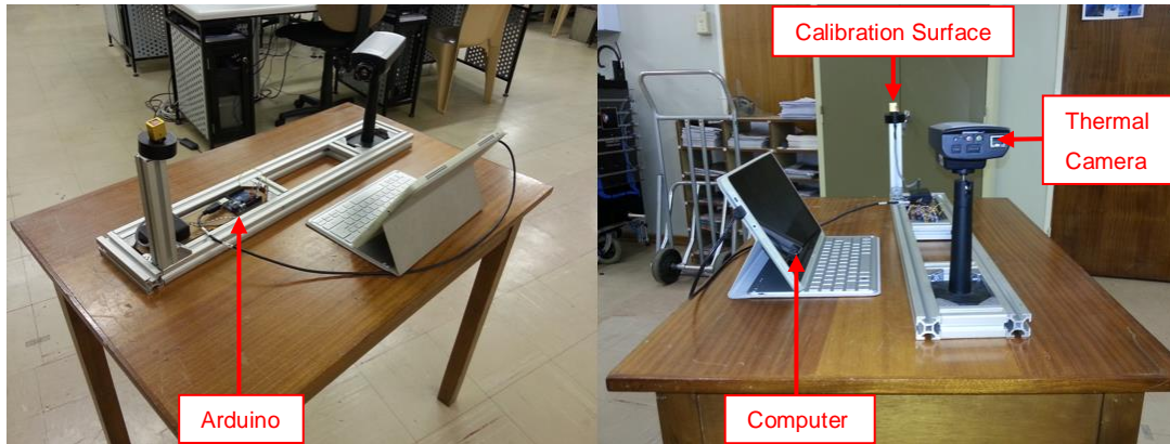
Figure 4-7 Thermal calibration setup overview
