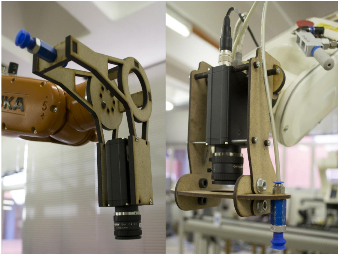
Figure 3.9 Cameras mounted as auxiliary tools
