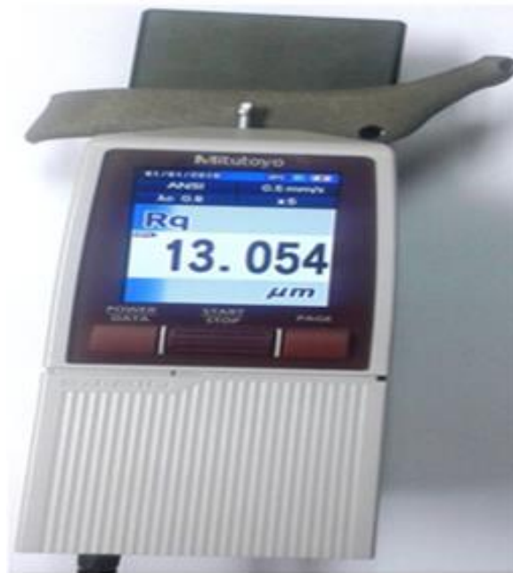
Figure 3.13: Root mean square ( R_q ) surface roughness of the implant as measured with SJ-210 roughness measuring device.
