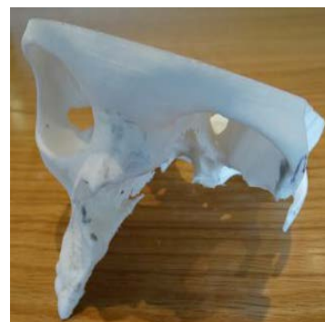
Figure 3 - Nylon model cut where the bone resection was planned
