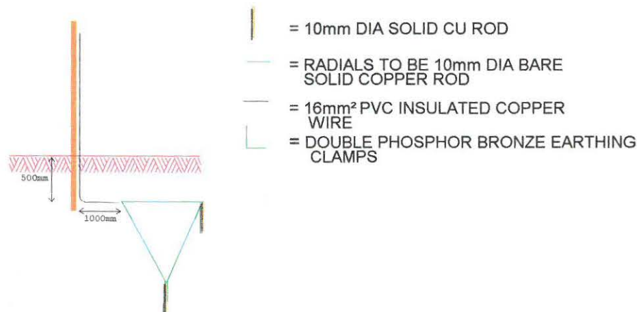
Fig. 5.12 Earthing Materials at Isolating Transformer
