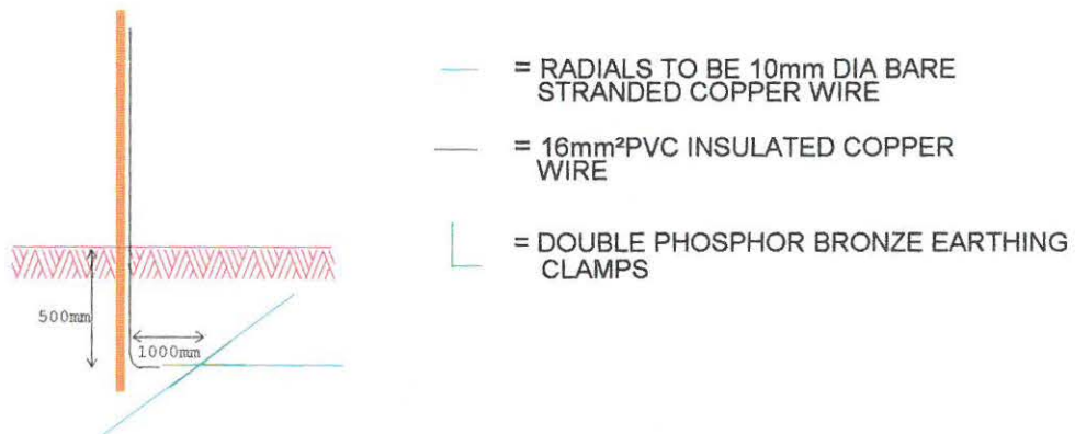
Fig. 5.14 Materials at Distribution Transformer Trench Earth Electrode
