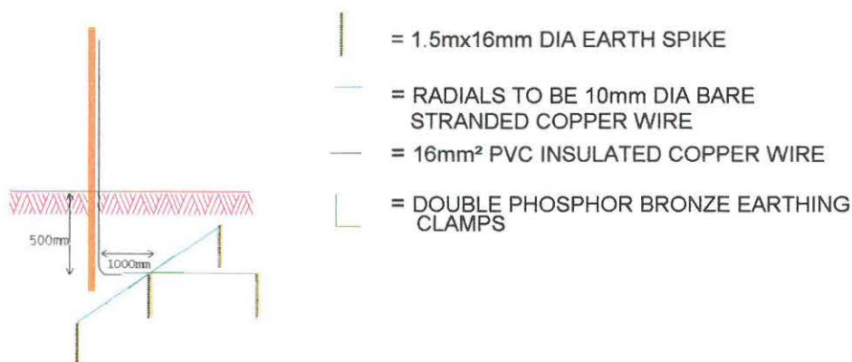
Fig. 5.13 Materials at Distribution Transformer Crowsfoot Earth Electrode
