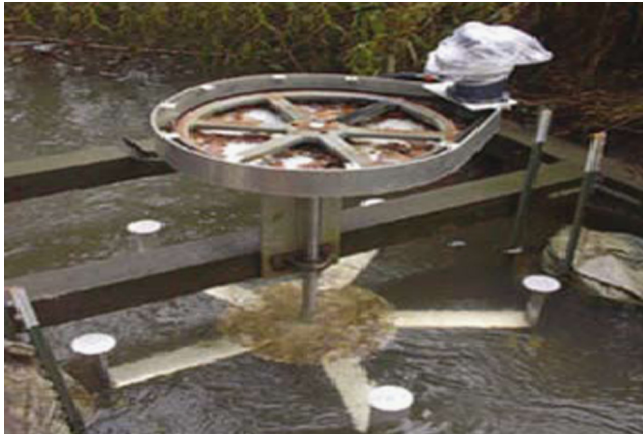
Fig. 3. Installed freestream Darrieus hydrokinetic turbine [38].
