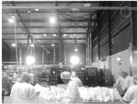
Figure 6: Image of the cameras and USB extender set above a line in the packaging department
