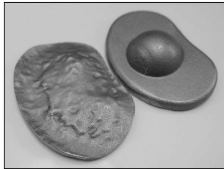
Figure 5 – An example of a patient-specific intervertebral implant manufactured from Ti6Al4V using Direct Metal Laser Sintering
