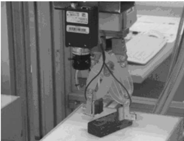
Fig. 3. Arrangement of camera and robot gripper
