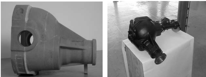
Figure 18: Differential Housing made with a 3DP Pattern and Investment Casting
