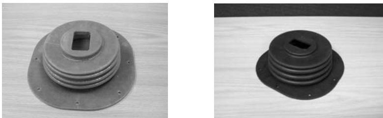
Figure 16: Rubber similar part built on a Z Corp 3D Printer (left); compression moulded rubber part (right) (courtesy of CAE – Stellenbosch Automotive Engineering)
