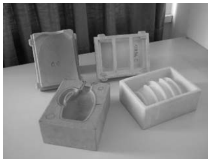
Figure 22: Wax patterns for investment casting with cooling channels and water jackets
