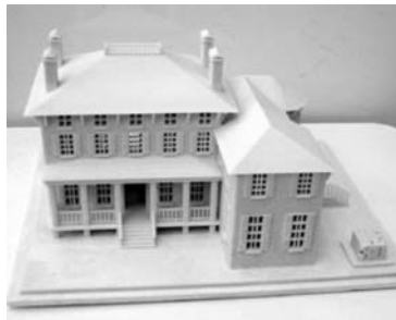
Figure 25: Architectural model printed in plaster based powder. Printing Time: 5.5 hours, dimensions: 200×240×120mm [35]
