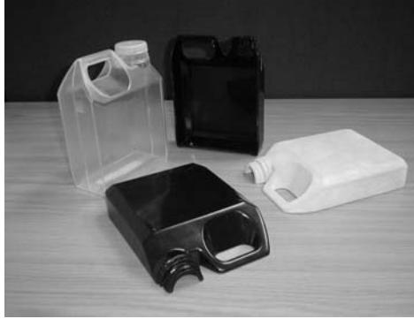
Figure 14: Transparent bottles produced for customer presentation. Uninfiltrated part and patterns are also shown [18]
