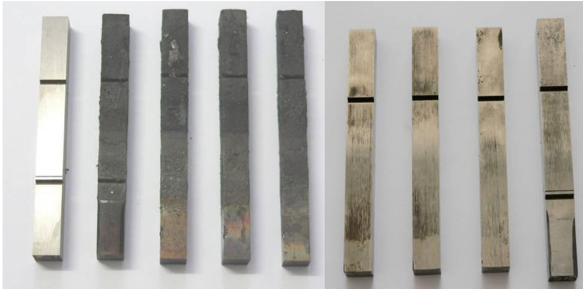
Figure 5.5 Specimens after and prior to 10 000 aluminium melt dipping cycles
