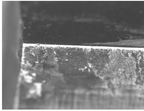
Al welding, and cracks (post 5 000 dips)
