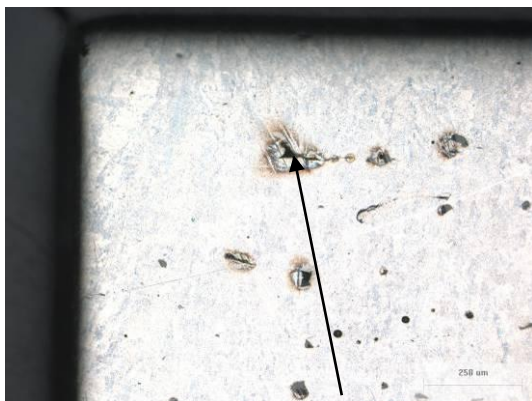
D2 clearly visible crack initiation
