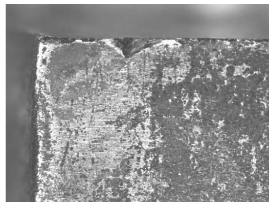
Al welding, pitting and cracks (post 5 000 dips)
