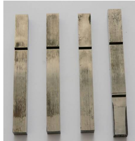
Figure 7.4 Specimens prior and after 10 000 aluminium melt dipping cycles
