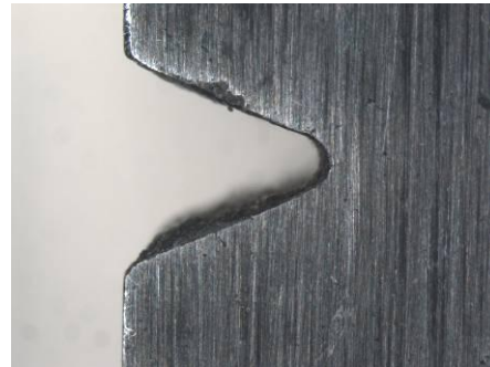
Notch after 10 000 dips. Note chipping, and washout
