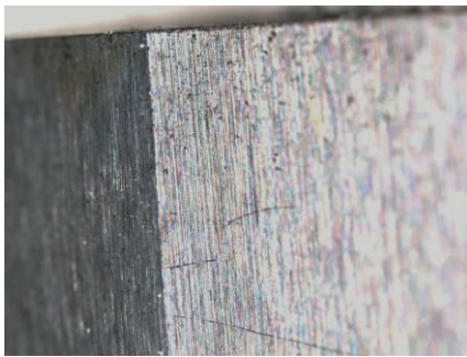
Typical corner aspect prior to dipping
