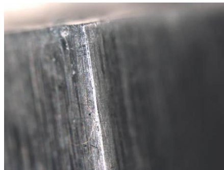
Al welding, pitting & wash (post 10 000 dips)
