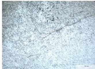
LENS microstructure very coherent due to the complete melting of powders during processing (200x). Hardness= 52 HRC
