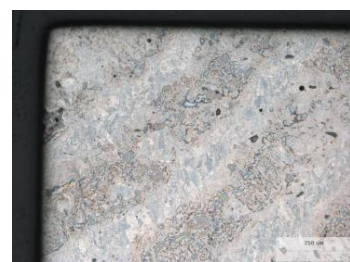
Concept coupon prior to dipping. Small number of pores visible (100x)
