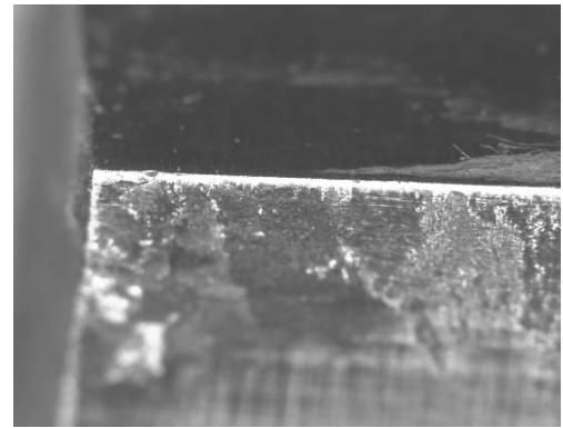
Al welding and cracks (post 5 000 dips)
