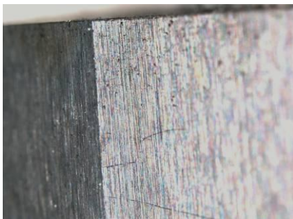
Typical corner aspect prior to dipping
