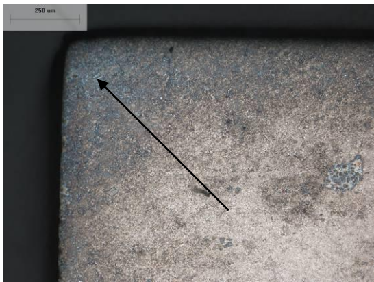
Notice oxidation emanating from corner of dipped H1 specimen due to decarburisation of the outer surfaces
