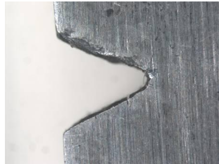
Notch after 10 000 dips. Not chipping, crack initiation and washout
