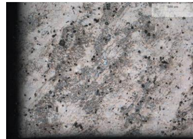
Concept coupon after dipping. Note agglomeration and segregation of intermetallic alloys coupled with increased number of small pores (200x).
