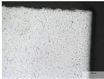
Typical aspect of sharp corner of LENS specimen prior to dipping (20x)
