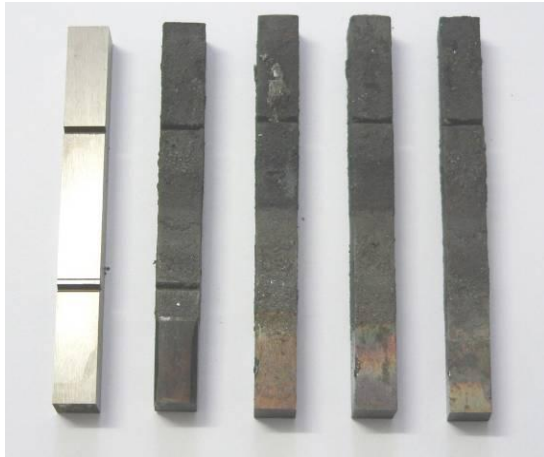
Figure 7.4 Specimens prior and after 10 000 aluminium melt dipping cycles
