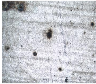
H13 microstructure after dipping (200x). Hardness = 45HRC. No significant variance on microstructure. Minor porosities and inclusions.
