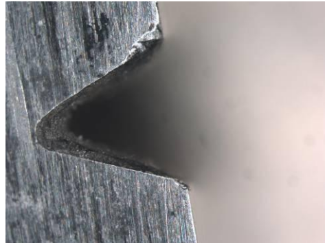
Al welding and cracks (post 10 000 dips)
