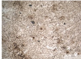
LENS specimen microstructure after dipping (200x). Hardness = 50HRC. No significant variance of matrix with minor porosities and inclusions.
