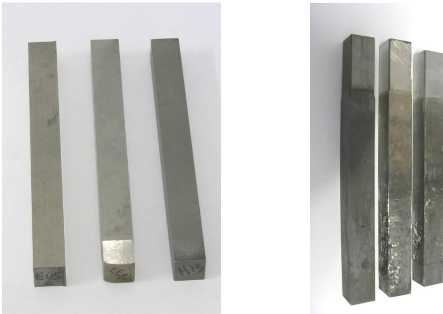
Figure 4.5 Specimens prior to and after 5 000 aluminium melt dipping cycles
