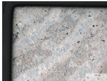
Concept specimen melt deposition tracks visible - nucleation and aggregation of intermetallic alloys (100x)
