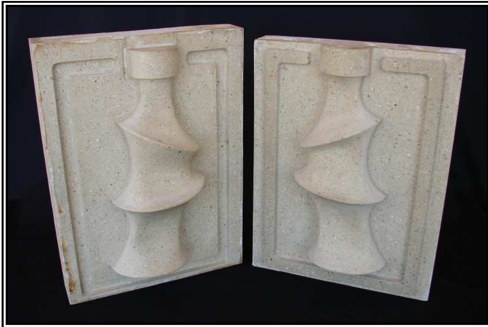
Figure 94: Lofted vessel 1: CNC milled vessel prototype
