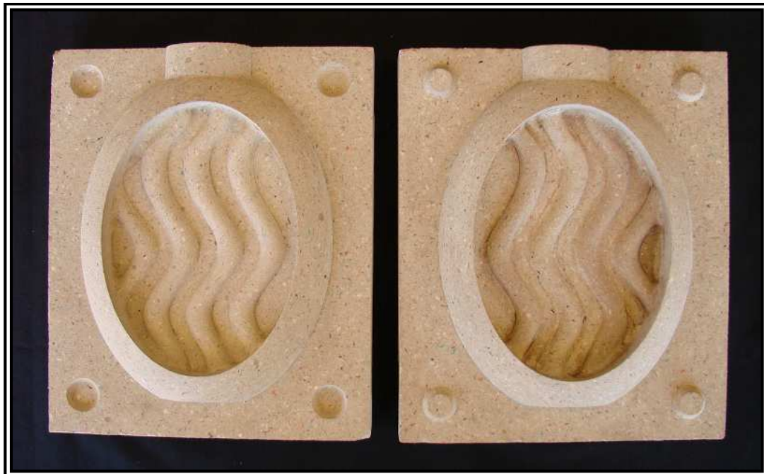
Figure 109: Swept vessel 2: CNC milled vessel prototype
