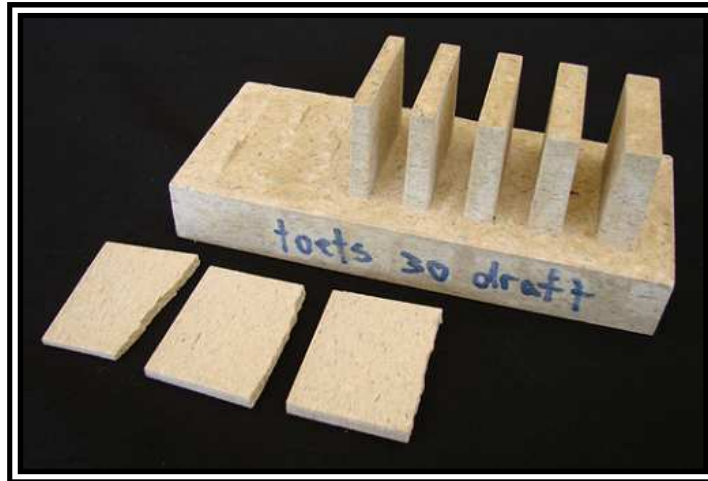
Figure 70: Test geometry 6 – CNC milling
