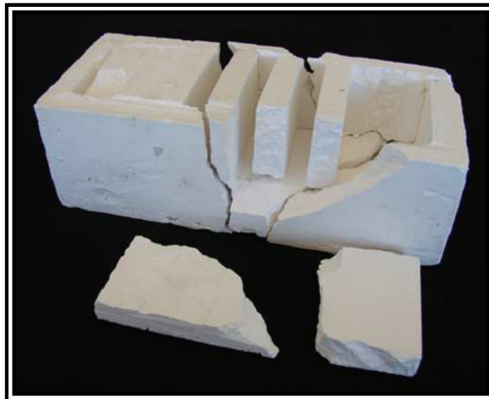
Figure 71: Test geometry 6 – test – plaster of Paris mould
