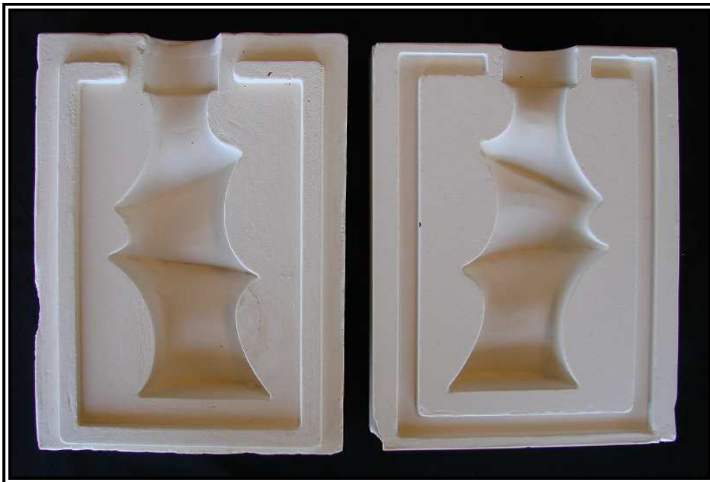
Figure 96: Lofted vessel 1: Plaster of Paris master mould
