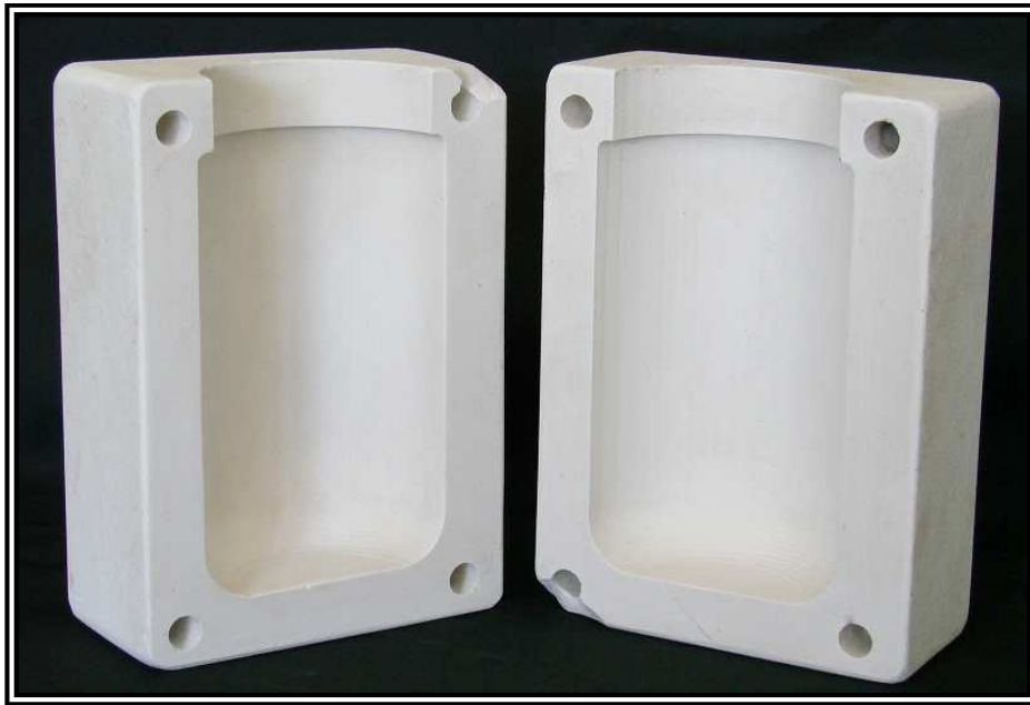
Figure 11: Direct CNC milled plaster of Paris test geometries, 168 mm x 120 mm x 55 mm
