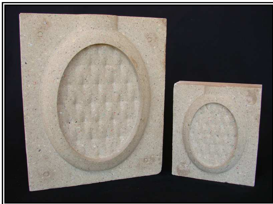
Figure 138: Solid mesh vessel 4: CNC milled vessel prototypes
