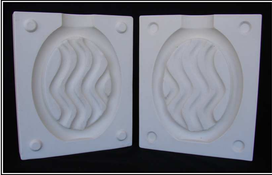
Figure 111: Swept vessel 2: Plaster of Paris master mould
