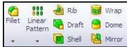
Figure 9: Diagram of operation-based features
