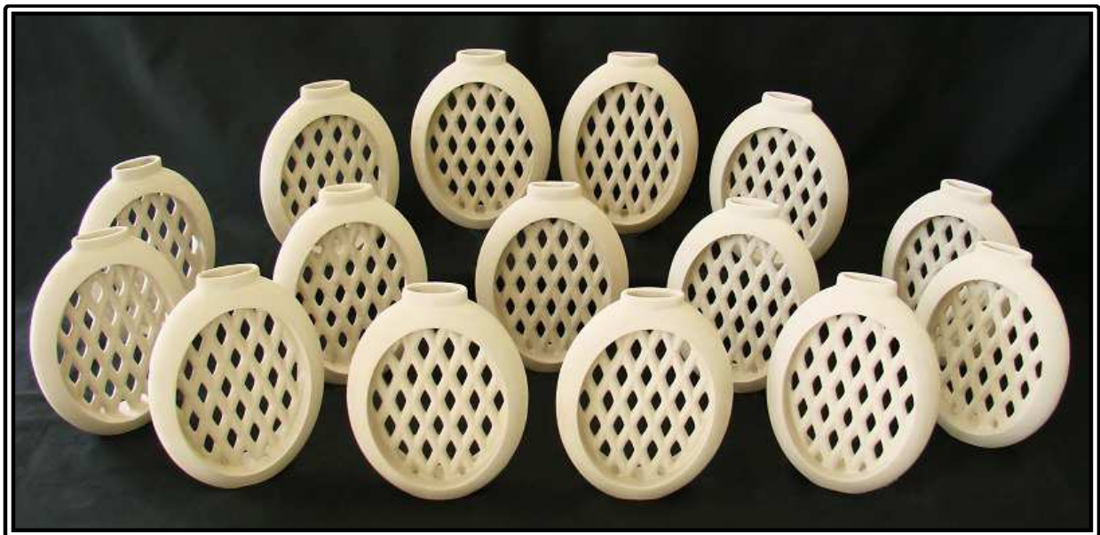
Figure 130: Mesh vessel 3: Batch production range of 15 units
