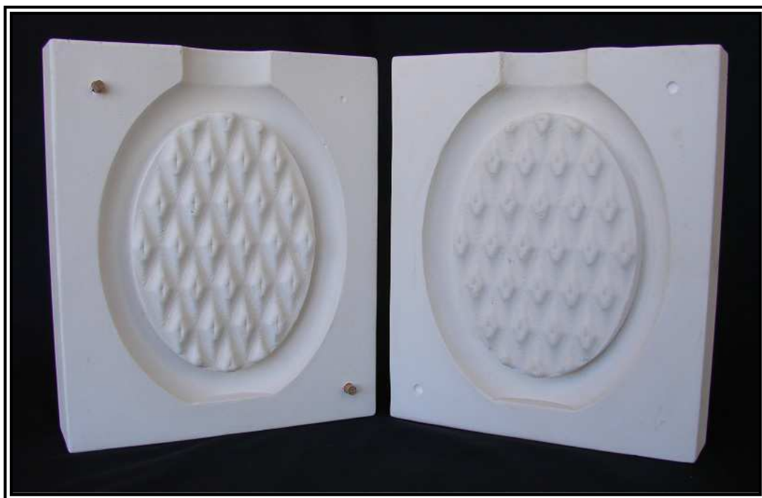
Figure 126: Mesh vessel 3: Plaster of Paris master mould
