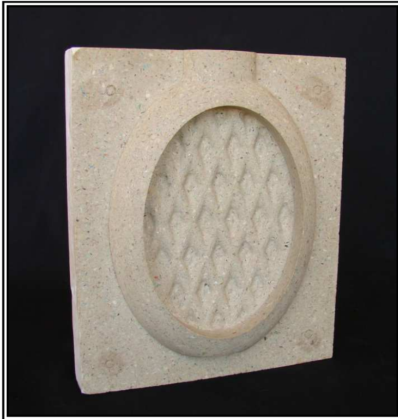
Figure 124: Mesh vessel 3: CNC milled vessel prototype
