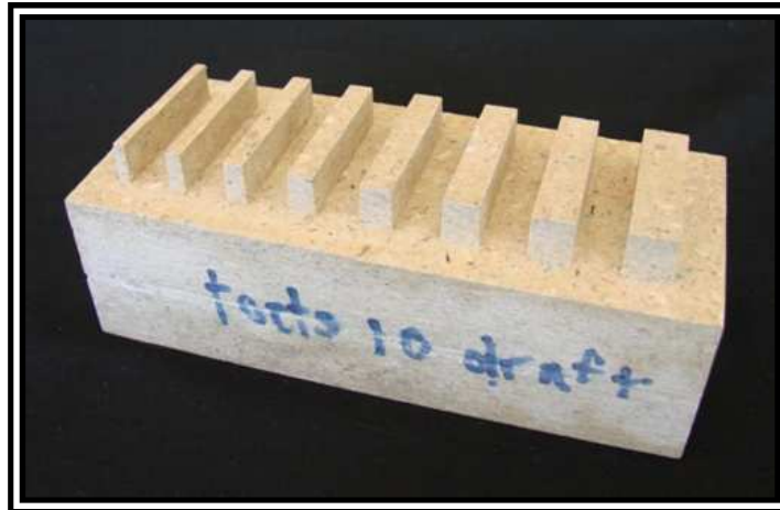
Figure 49: Test geometry 2 – CNC milling
