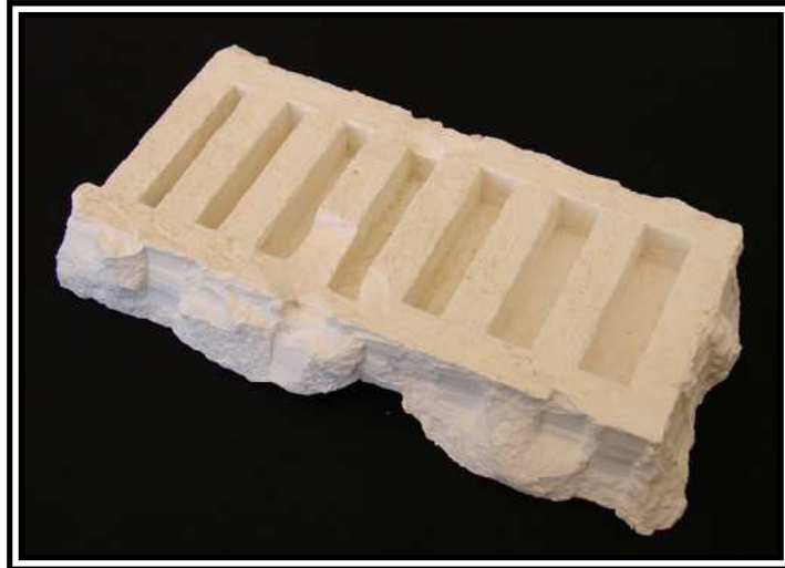
Figure 45: Test geometry 1 – plaster of Paris mould
