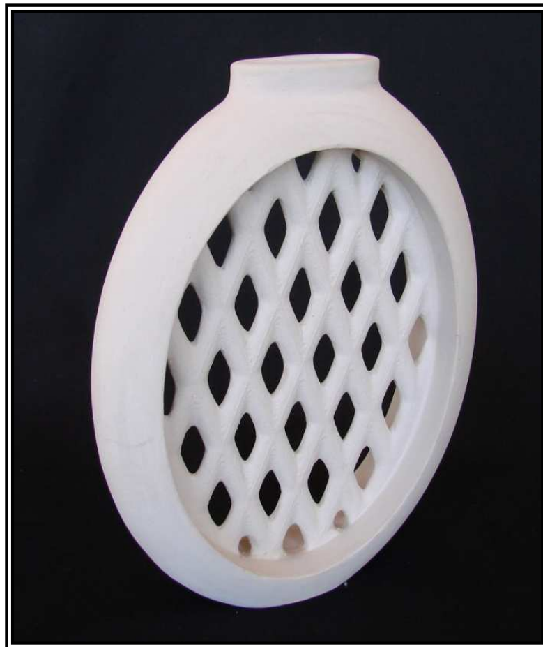
Figure 128: Mesh vessel 3: Final slipcasting vessel
