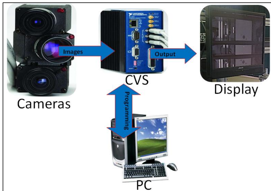
Figure 3.13: Vision System Component Relationship
