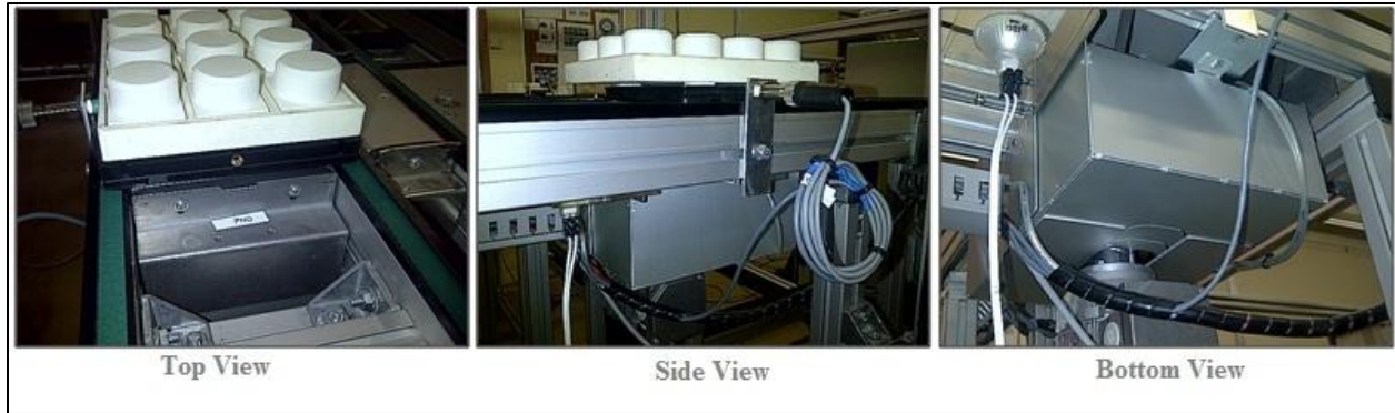
Figure 3.12: Mechanical Structure of the Conveyor System at the Point of Inspection
