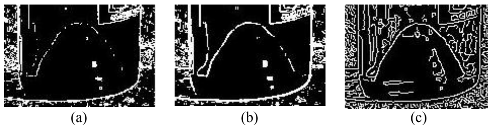
Figure 2.11: Results obtained by utilising different operators viewing only a section of the image used in Figure 2.10(a) – (a) Roberts operator result; (b) Prewitt operator result; (c) Canny edge result
