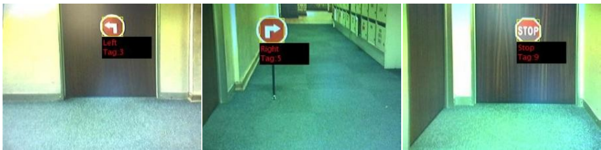
Figure 4.38: Displayed recognised left, right and stop signs
