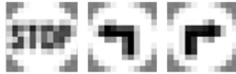
Figure 4.35: Three signs template, generated for the detection process, STOP, left and right turn
