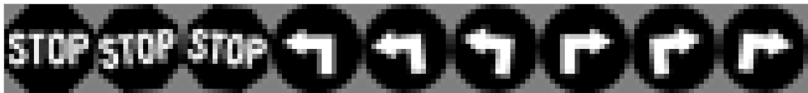
Figure 4.36: Three signs templates – STOP, left and right; with three orientations each, 0^\circ + 7.5^\circ and -7.5^\circ ; generated for recognition process
