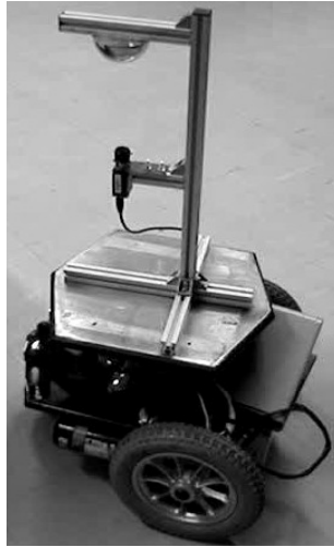
Figure 2.5: AGV with hyperbolic mirror setup
