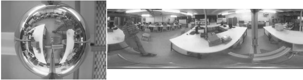
Figure 3.11: Transform with image facing the front not centred, but mirror image effect corrected already
