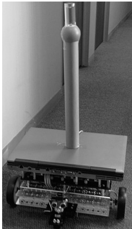
Figure 4.6: AGV platform utilising a laptop, NI robot platform and omnivision system
