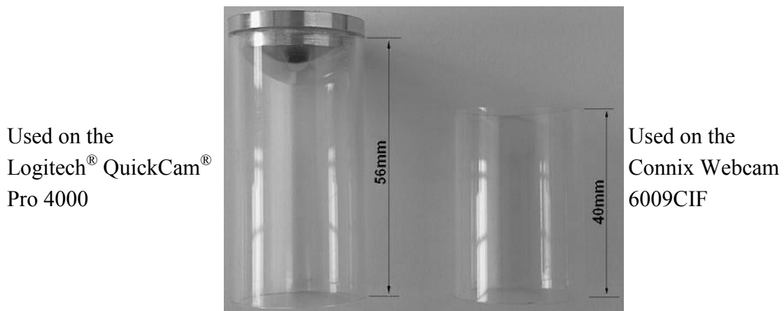
Figure 5.1: Mirror and different Perspex® tubing lengths for webcam setup
