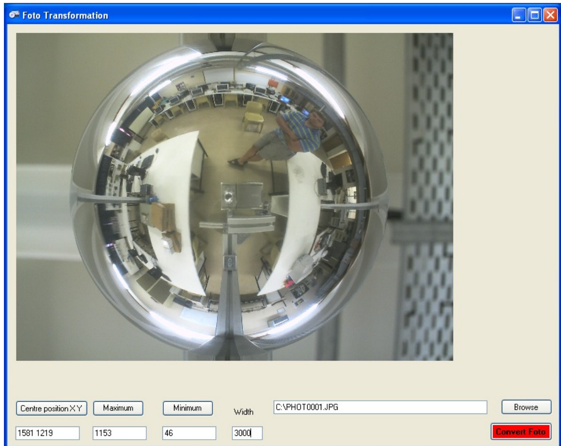
Figure 3.13 C# developed GUI utilising a transformation exe-file compiled from a MATLAB ® M-file
