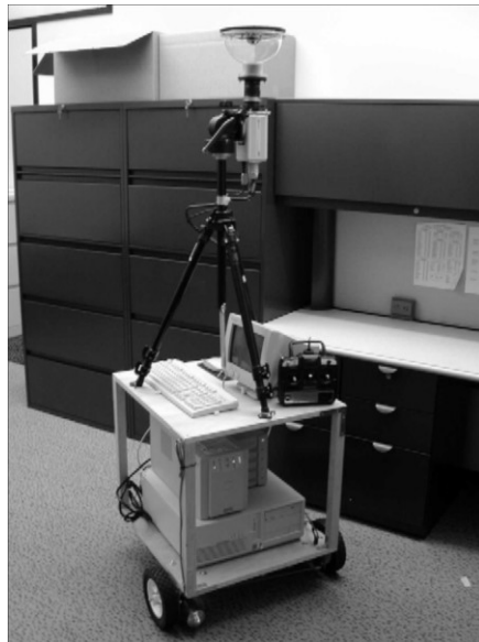
Figure 2.8: Camera setup of Aliaga with parabolic mirror and acrylic half sphere on a video camera [11]
