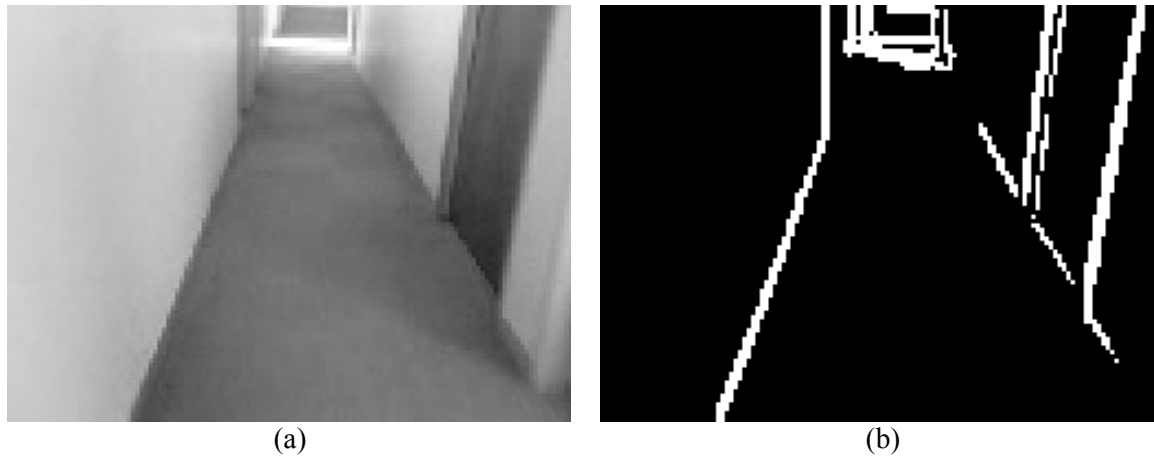
Figure 4.10: (a) Frame captured from a colour camera; (b) Prewitt edge detection applied on a frame
