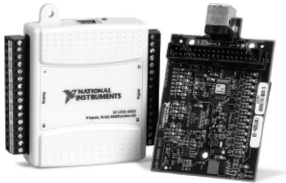
Figure 4.25: NI USB-6009 inside and outside its enclosure
