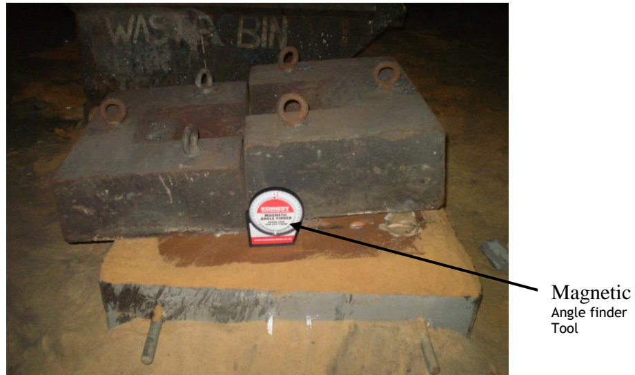
Figure 6.3 Assembled mould with weights and required inclination (see magnetic angle finder tool) ready to be poured.
