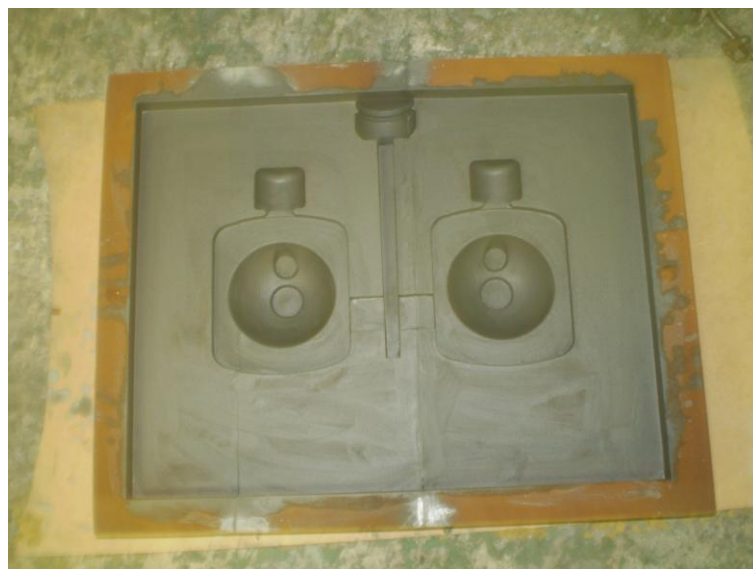
Figure 6.2 Drag component of the mould with the internal cavity of the tool to be cast.
