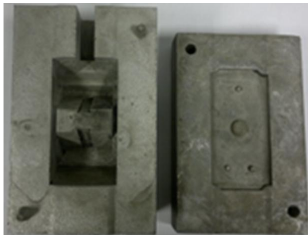
Figure 9.3 (a) CAD of the lower part of the die, (b) DC mould, (c) RCT die before finishing operations
