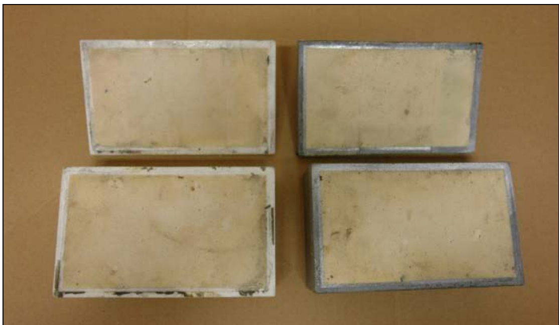
Figure 4.43: The filled second mould sintered in polyamide and Alumide®
