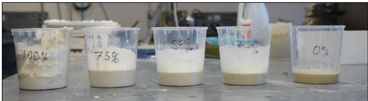
Figure 4.13: Powder/resin mixture test pieces
