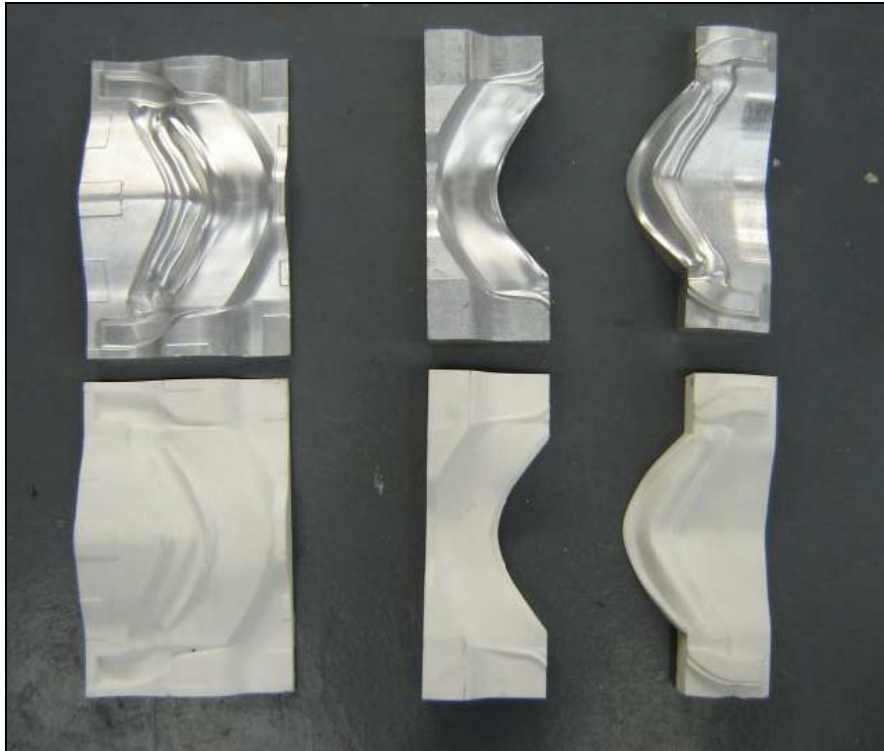
Figure 4.19: Comparison between the sintered mould and the aluminium CNC mould
