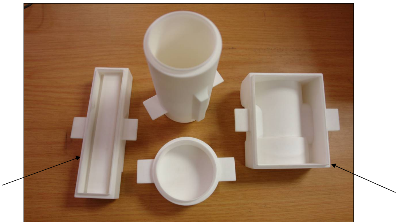
Figure 4.36: The 5 mm extrusion on the back of the part and the ears to assist with machining
