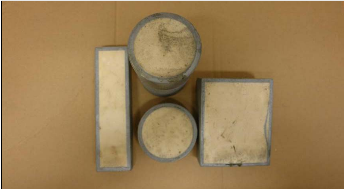
Figure 4.38: The Alumide® mould with filled back
