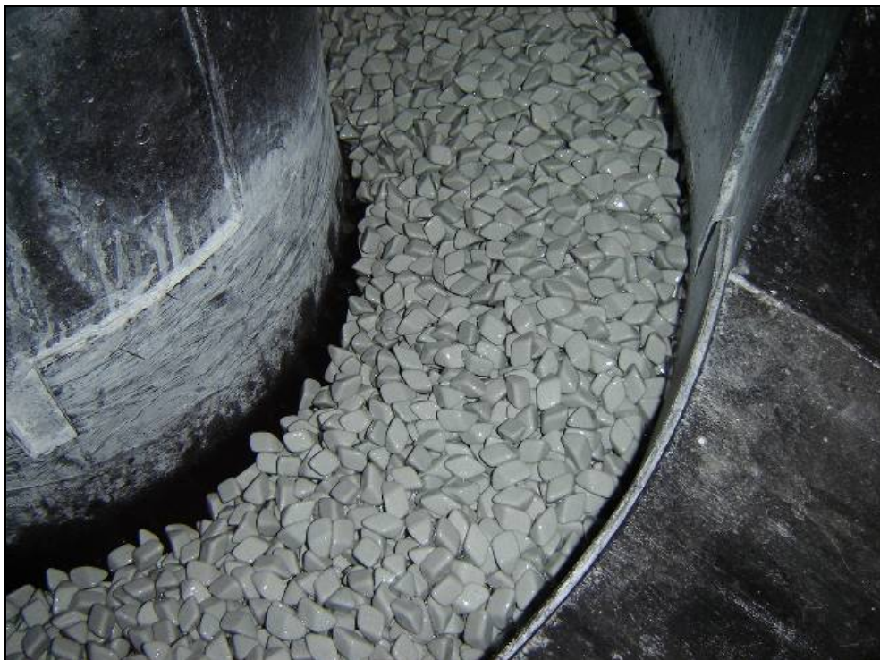
Figure 4.35: The abrasive stones in the vibrating machine
