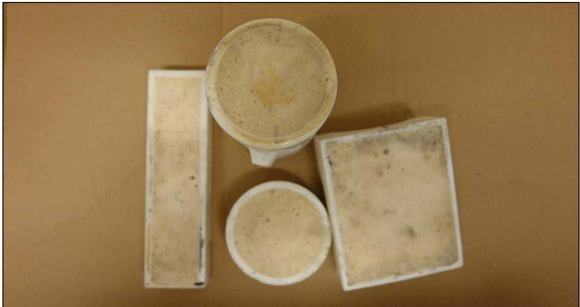
Figure 4.37: The polyamide mould with filled back
