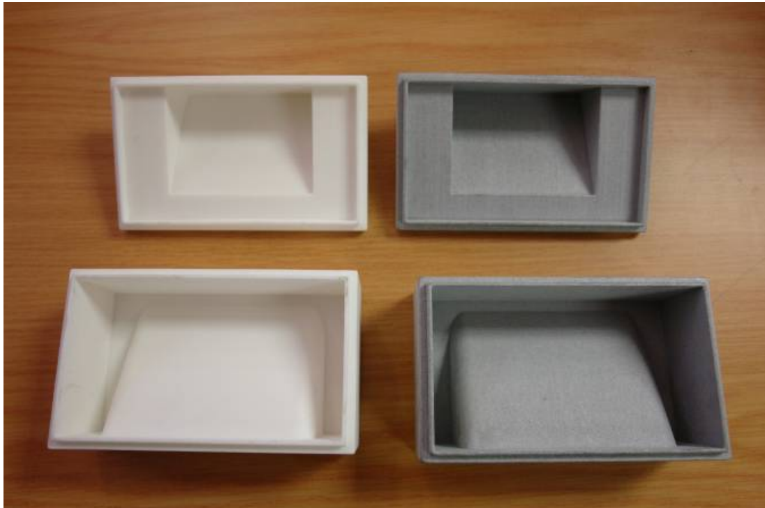
Figure 4.42: A bottom view of the second mould sintered in polyamide and Alumide®
