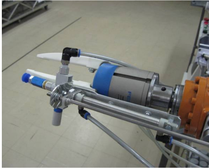
Figure 3-5 Extensible suction cup model 1
