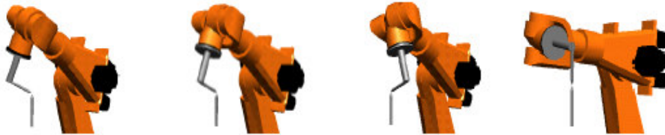
Figure 4-14 Four-point calibration method [4]
