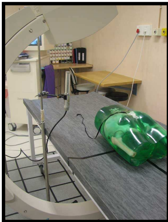
Fig. 3.15 C-Arm in Oblique position with the Berthold probe on a drip stand
