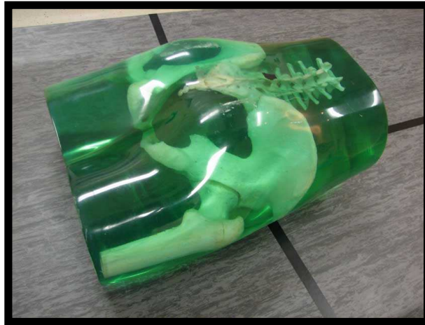
Fig. 3.10: Perspex phantom for measurements to simulate a patient
