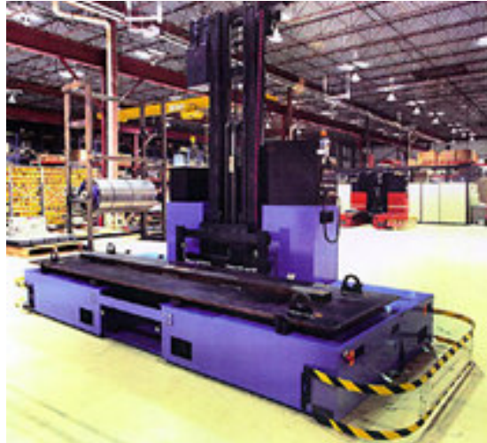
Figure 1.1: AGV used in an airplane-manufacturing plant
