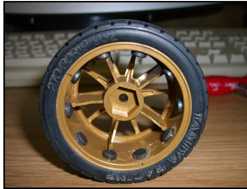
Figure 3.10: Wheel of AGV with magnets on
