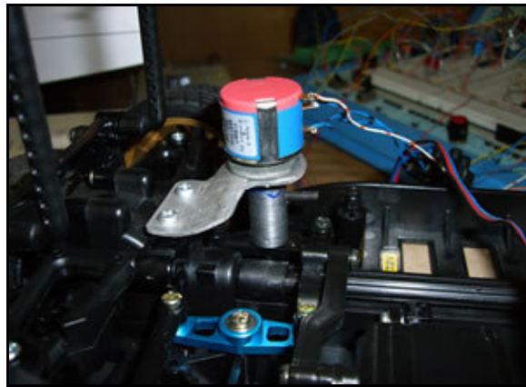
Figure 3.15: Precision potentiometer for steering control
