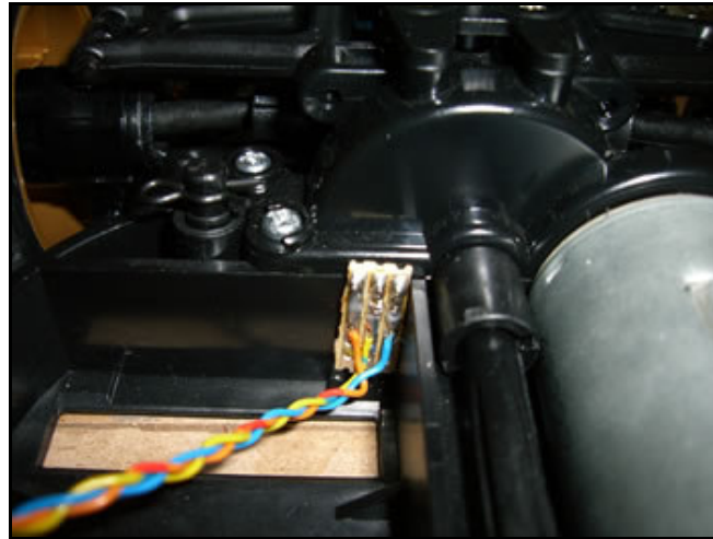
Figure 3.12: Hall-effect sensor mounted onto gearbox
