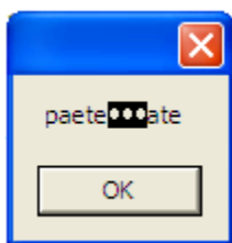
Figure 5.1: Output of a captured word and the effect when the internal representation of certain keyboard keys is not handled by the software, in this case, the backspace key in particular
