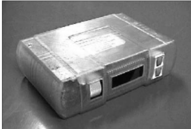
Figure 12-4: The final SLA product
