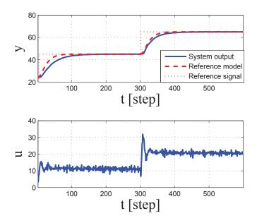
Figure 3.19: Experimental control performance using CMAC-FRIT-PID controller for untrained signals  $\$
