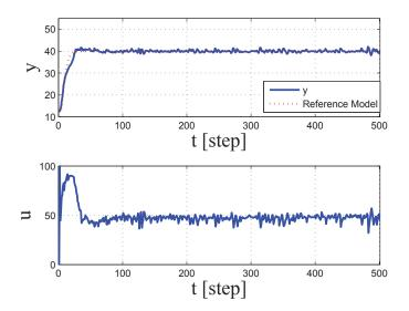
Figure 4.23: Control performance of CMAC-PD-FRIT-PID controller
