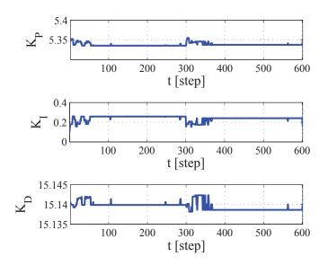
Figure 3.20: Trajectories of controller gains using proposed method for untrained signals
