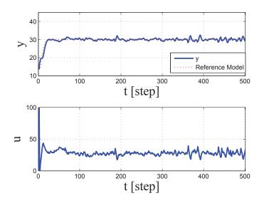
Figure 4.28: Control performance for untrained signal using HC-CMAC-PD-FRIT-PID controller
