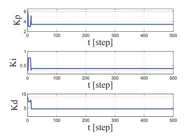
Figure 4.26: Trajectories of PID gains using HC-CMAC-PD-FRIT-PID controller
