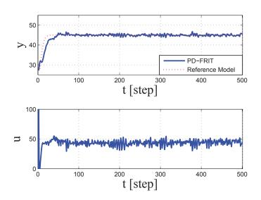
Figure 4.18: Control performance using PD-FRIT-PID method
