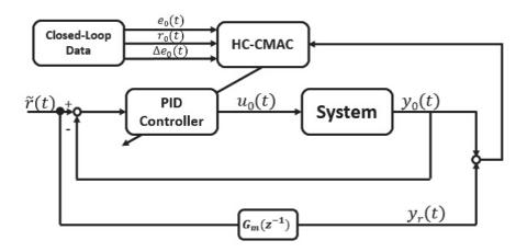
Figure 3.2: Block diagram of HC-CMAC-FRIT
