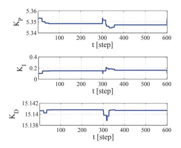
Figure 3.21: Trajectories of controller gains using CMAC-FRIT-PID controller for untrained signals
