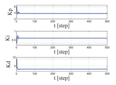
Figure 4.25: Trajectories of PID gains using CMAC-PD-FRIT-PID controller in Fig. 4.27 and Fig. 4.28. In the transient state, the integral absolute error(IAE) of CMAC-PD-FRIT-PID is 85.32, the IAE for HC-CMAC-PD-PID controller is 45. It demonstrated that the HC-CMAC-PD-FRIT-PID
