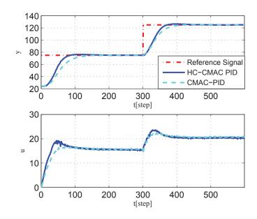
Figure 2.23: Control performances of CMAC with 3 weight tables 8 labels and HC-CMAC-PID controller
