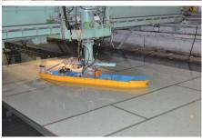
Figure: Experiment in shallow water (Hiroshima University towing tank)
